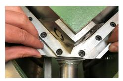
The fixed bottom blades should be a smooth sliding fit against the moving blades. make a test cut using a sheet of copier paper or similar.
