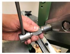
8. Adjust the bottom blades away from you so that they just meet the top blades. Start at the front and work your way towards the back while raising the blades with the foot pedal.
