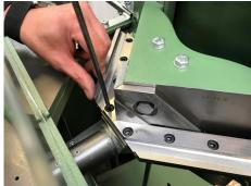
3. On each side, loosen and remove the bolts. First the top and bottom ones. Finally the middle bolt and carefully lift the blade and place it on a safe surface.
