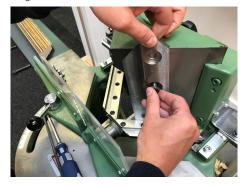
6. Using a large, flat-bladed screwdriver (never a hammer!) carefully adjust the positions so that the bottom edges of the blades are aligned. The point where the blades meet at the front should be flush, with neither standing proud.
