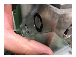
7. Fully tighten the bolts in the upper blades.
